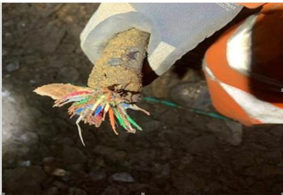
In the early hours of Sunday 11<sup>th</sup> October Network Rail contractors working on the drainage at Melksham Station damaged a cable. Signalling records did not indicate the presence of the cable and it was thought it was no longer in use. However when the line was re-opened to trains just over 24 hours later it was discovered that some of the signalling was not working and services were disrupted.
